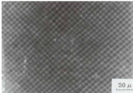
Figure 9. Square lattice pattern above E_C in zone 6. E = 2.0 \times 10^6 V/m; f = 800 Hz.
